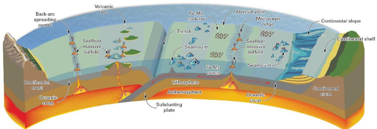
**Figure 4 A cross-section through the Earth's crust showing the different types of plate boundary, the topography of the ocean floor and the distribution of the major metal-rich deep ocean mineral deposits**
